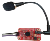
Gambar 3 . Modul Voice Recognition V3
